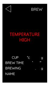
If brewing temperature is lower than water in boiler, "TEMPERATURE HIGH" message displays.
