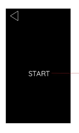
If you touch the start button, water in the boiler drains away and it will automatically change to a stop button.
